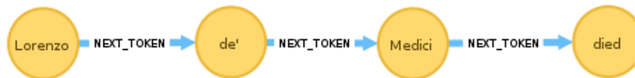
Fig. 10: Text as a chain of word nodes in the Neo4j browser. [Neill / Kuczera 2019]
