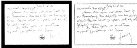
figure 3: Binarization examples obtained from Otsu's method (left) and obtained from Bradley's method (right).
