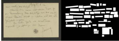
figure 2: Text detection mask (left), overlaid with the binarized input image to generate the contours (right). Local feature descriptors are extracted at the contours and aggregated to form a global image descriptor.
